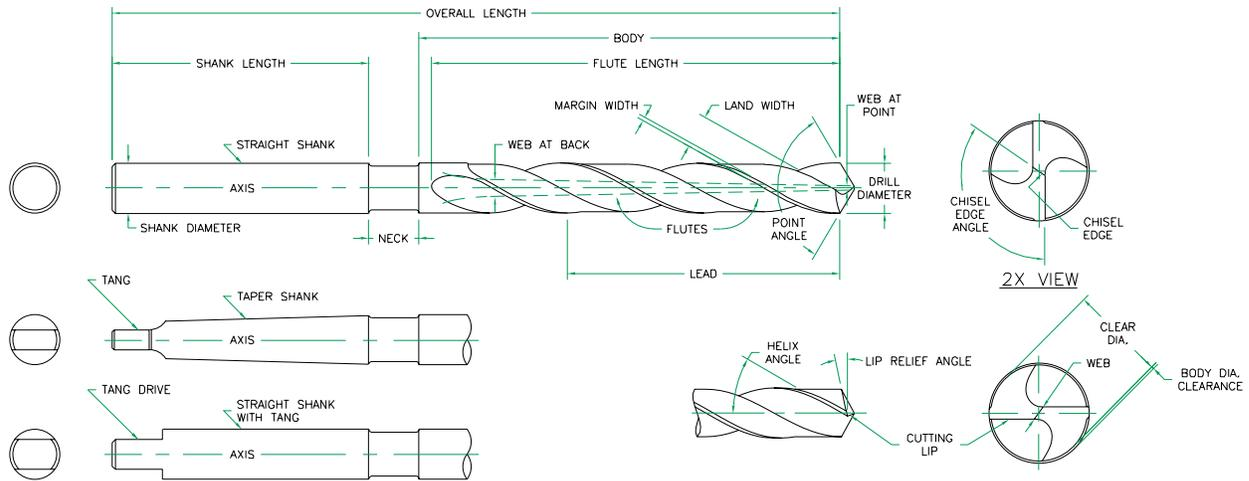
**Axis**—The imaginary straight line which forms the longitudinal center line of a drill.
